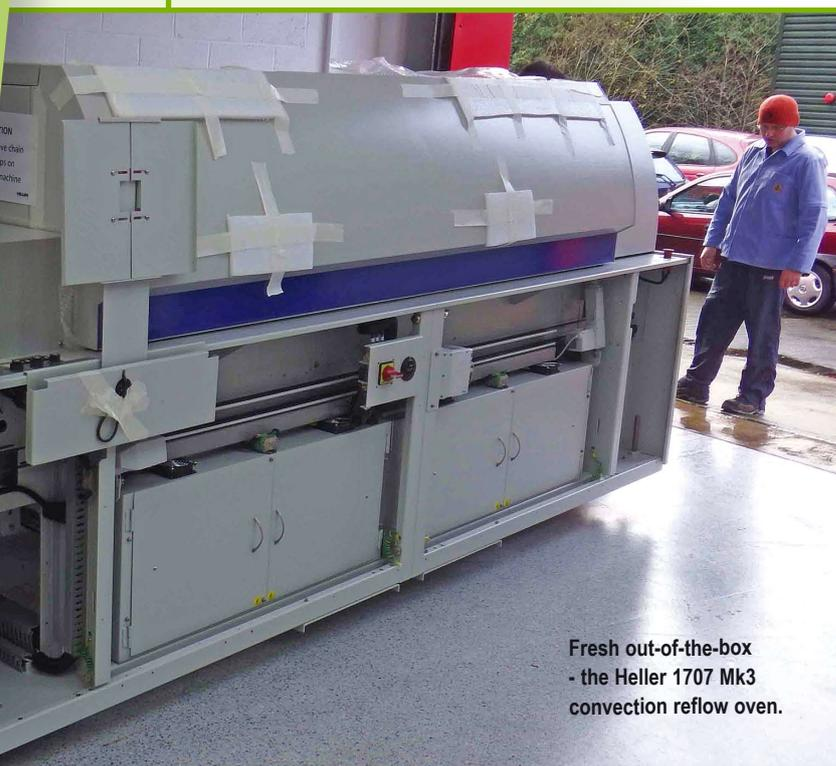
Fresh out-of-the-box - the Heller 1707 Mk3 convection reflow oven.
