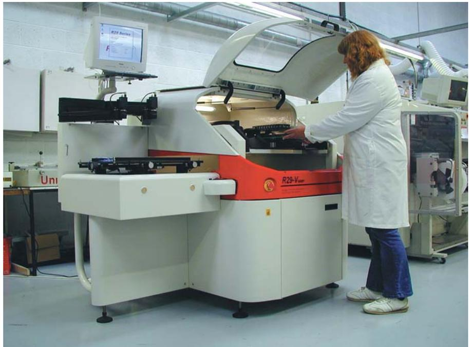
Vision alignment control on this newly installed machine enables very accurate solder paste printing and increases product reliability.
