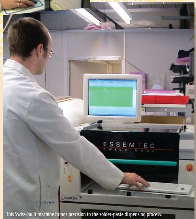
This Swiss-built machine brings precision to the solder-paste dispensing process.
