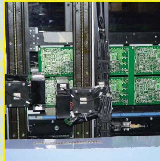
Performance and efficiency are greatly enhanced with the installation of a second electrical testing machine.
