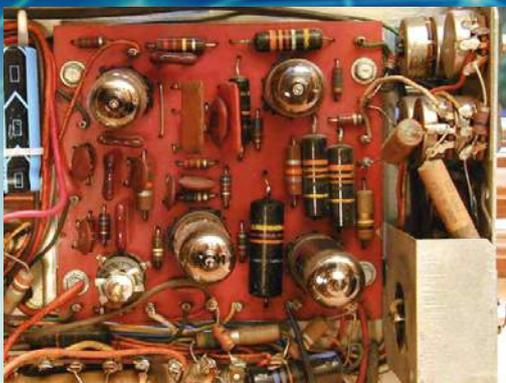
A selection of typical 1950s circuit boards. Notice the valves (vacuum tubes) in the picture above. All parts were placed and soldered by hand.
